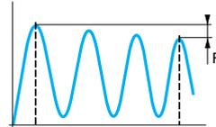
The tolerance of the switching point throughout the entire service life of the switch.
