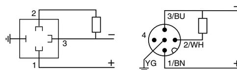
(2) Switch connector pin view
