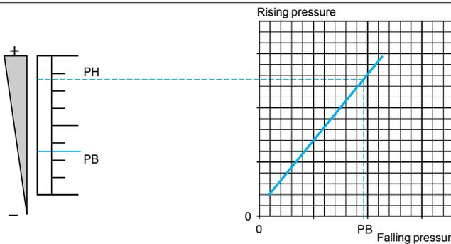
The pressure at which the switch contact changes state, for each stage, on falling pressure.
