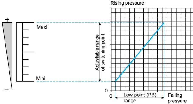
Defined by the difference between the minimum and maximum high point (PH1 or PH2) setting values for each stage.
