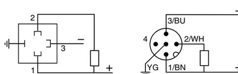
(1) Sensor connector pin view
