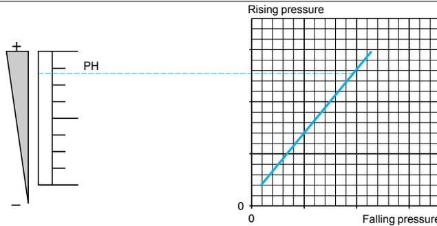
The upper pressure setting at which the pressure or vacuum switch will actuate the contact, for each stage, on rising pressure.
