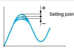
The tolerance between the point at which the switch actuates its contacts and the value indicated on the setting scale. Where very high setting accuracy is required (initial installation of the product), it is recommended to use separate measuring equipment (pressure gauge, etc.).
