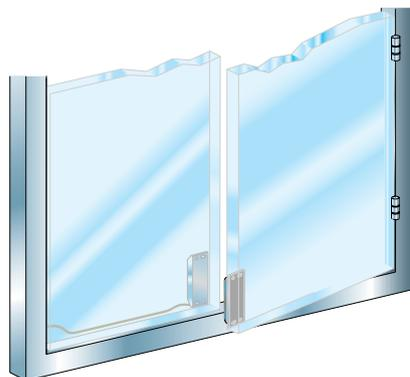
These switches provide a solution for monitoring moveable machine guards fitted to machines with quick rundown times. They are particularly suitable for guards without accurate guidance and for use in difficult environments (dust, liquids, etc.). Installing self-contained coded magnetic systems provides an optimum solution (no control system required). They enable:
