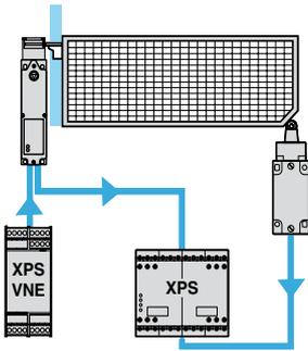
Interlocking device for actuator fitted on guard and zero speed detection.
