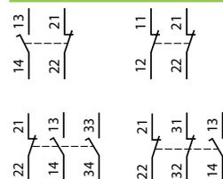
Safety switches **XCS PL** and **XCS PR** incorporate a 2-pole or 3-pole contact block, with positive opening operation. The contact arrangements can be: NC + NO break before make, 2 NC, 1 NC + 2 NO break before make or 2 NC + 1 NO break before make.
