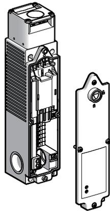
With the machine guard closed and locked, the resistance to forcible withdrawal of the actuator fitted to the guard is **Fzh 1100 N** according to the verification principle GS-ET 19 ( $F_{zh} = F_{max}/1.3$ ) with  $F_{max} = 1400N$ . In addition to the 2-pole or 3-pole contact block, positively operated by the actuator fitted to the guard, the switches incorporate **1 or 2 NC contacts mechanically linked to the solenoid**. The NC contact(s) are for use in the safety circuit of the machine.
