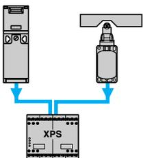
Locking of actuator and operation in positive mode associated with a safety module.
