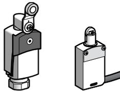
Metal or plastic case limit switches. For use on machines with low inertia and also on machines with high inertia, when used in conjunction with actuator operated guard switches, for monitoring access doors and/or guards. When used on their own, they are always installed in "positive mode" or combined in pairs, with one switch being in "positive mode" and the other in "negative mode".
