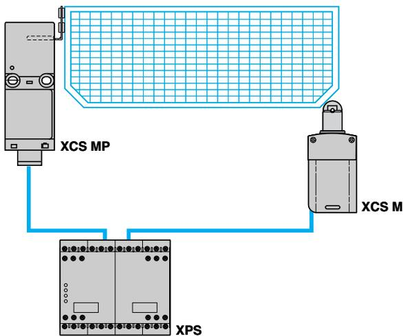
Locking of actuator and operation in positive mode associated with a safety module.
