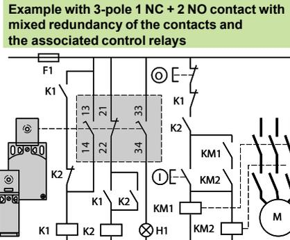
To activate K1, the lever or spindle must be rotated
