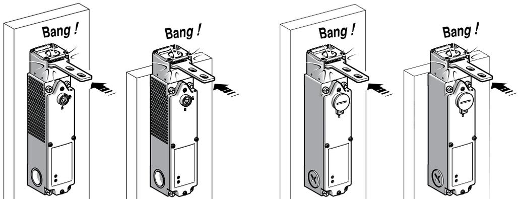
**Example of operation for an XCS LE key operated switch with locking on de-energisation of solenoid**
