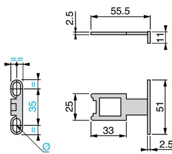
(1) Adaptor (included with actuator XCS Z01) for replacing, without drilling additional fixing hole, a guard switch XCK J with actuator ZCK Y07 by a guard switch XCS A, B, C or E with actuator XCS Z01.
