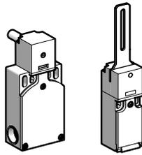
Plastic case guard switches with straight or elbowed operating lever or spindle operator. Specifically designed for small industrial machines fitted with small sized **hinged doors, covers or protective guards**. They protect the operator by immediately stopping the dangerous movement of the machine as soon as the rotary lever or spindle displacement reaches an angle of 5°.
