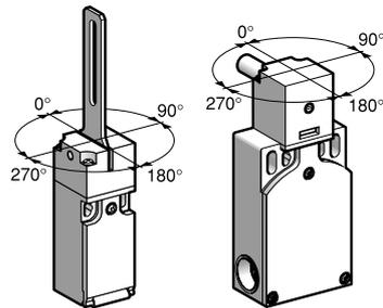
Safety switches for hinged covers or guards, featuring a hinged lever or spindle operator, incorporate a turret head that can be rotated through 360° in 90° steps. Two additional self-locking screws are included with each switch for positive fixing of the head.
