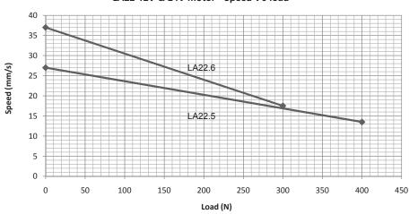
LA22 12V & 24V motor - Speed v's load
