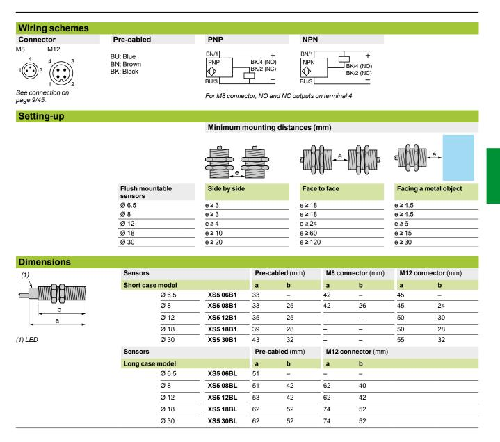
**Inductive proximity sensors** OsiSense XS, general purpose Cylindrical, standard range, flush mountable Two-wire DC
