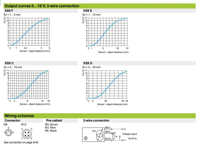
Output<br/>currentLoad impedance<br/>valueOutput<br/>voltageLoad impedance<br/>value24 V0...10 mA $R \le 1400 \Omega$ 0...10 V $R = 1000 \Omega$ Note: Ensure a minimum of 5 V between the + (terminal 1) and the sensor output (terminal 4).
