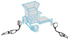
These inductive proximity sensors are designed for monitoring rotational speed or the speed of the flow of objects to be protected or monitored. They operate on the principle of comparing a speed threshold preset by the operator against the instantaneous measurement of the speed of the moving object to be
