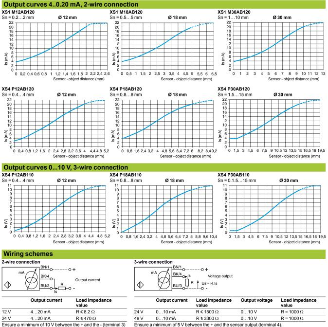
Ensure a minimum of 10 V between the + and the - (terminal 3) of the sensor.
