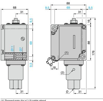
(1) Tapped entry for  $n^{\circ}$  13 cable gland (2) Drainage hole, tapped G 1/8 (female) Ø: G 3/8 (female)
