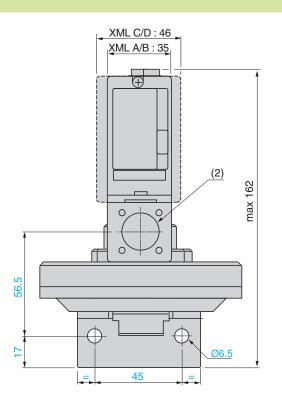
(1) 1 fluid entry, tapped G 1/4 (BSP female) (2) 1 electrical connections entry, tapped M20 x 1.5 or Pg 13.5
