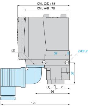
(1) 1 fluid entry, tapped G 1/4 (BSP female) (2) 1 electrical connections entry, tapped M20 x 1.5 or Pg 13.5
