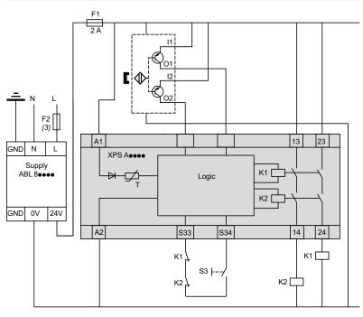
(1) The K1 and K2 coils must be protected with arc suppressors.
