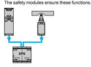
Locking of actuator and operation in positive mode associated with a safety module.
