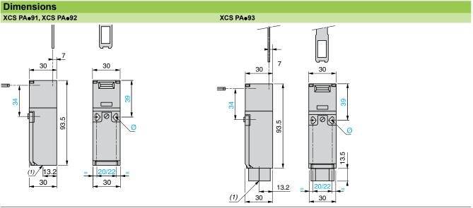
(1) 1 tapped entry for cable gland Ø: 2 elongated holes Ø 4.3 x 8.3 on 22 centres, 2 holes Ø 4.3 on 20 centres
