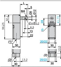
(1) 1 entry tapped for n° 11 cable gland (2) 1 entry tapped for 1/2" NPT conduit longated holes Ø 4.3 x 8.3 on 22 centres, es Ø 4.3 on 20 centres L = 30 (XCS PR•5•) or 80 (XCS PR•6•)
