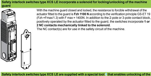
With the machine guard closed and locked, the resistance to forcible withdrawal of the actuator fitted to the guard is Fzh 1100 N according to the verification principle GS-ET 19 (Fzh =Fmax/1.3) with F max = 1400N. In addition to the 2-pole or 3-pole contact block, positively operated by the actuator fitted to the guard, the switches incorporate 1 or 2 NC contacts mechanically linked to the solenoid.
