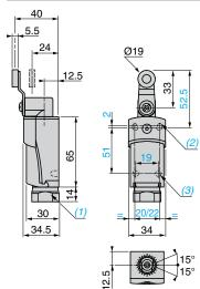
(1) Tapped entry for ISO M20 x 1.5 or Pg 13.5 cable gland or tapped 1/2" NPT.
