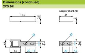
(1) Adaptor (included with actuator XCS Z01) for replacing, without drilling an additional fixing hole, a guard switch XCK J or XCS L with actuator ZCK Y07 with a guard switch XCS LF with actuator XCS Z01.
