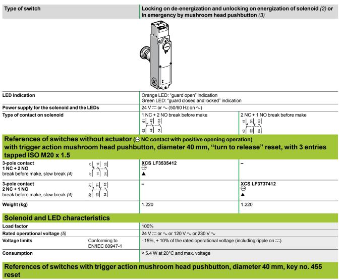
To order a switch with trigger action mushroom head pushbutton, key no. 455 release, diameter 40 mm at the rear of the product, replace the 5<sup>th</sup> number in the selected reference with **6**.
