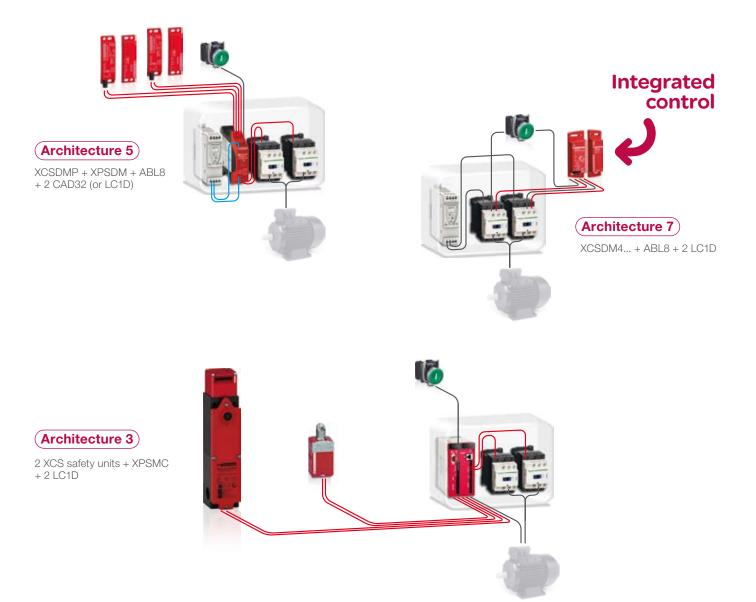
Used with Preventa modules, controllers or safety PLCs and TeSys motor starter solutions, XCS safety switches offer levels of access protection up to PLe, category 4, SIL3, according to standards requirements in force EN ISO 13849-1 and EN/IEC 62061.
