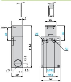
(1) 2 tapped entries for cable gland or 1/2" NPT conduit adaptor (2) 2 elongated holes Ø 4.3 x 8.3 on 22 centres, 2 holes Ø 4.3 on 20 centres
