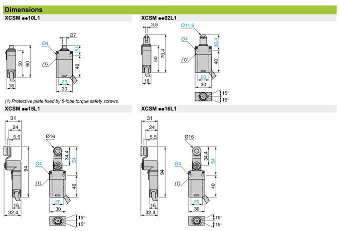
(1) Protective plate fixed by 5-lobe torque safety screws.
