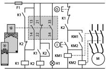
To activate K1, the lever or spindle must be rotated when the supply is switched on. H1: "lever or spindle displaced from initial position" indicator. When used in conjunction with an XPS module and another safety switch, the rotary lever or spindle operated switch can provide locking protection to PL=d, category 3 or PL=e, category 4 conforming to EN/ISO 13849-1.
